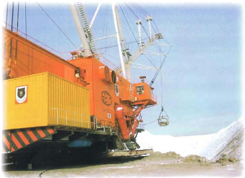
Dragline ESH 90/15 - main hoist drive equipped with electrohydraulic disc brakes operated by ELHY®-thrusters
