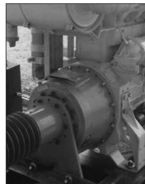
Wichita PTO mounted on Caterpillar diesel engine.
