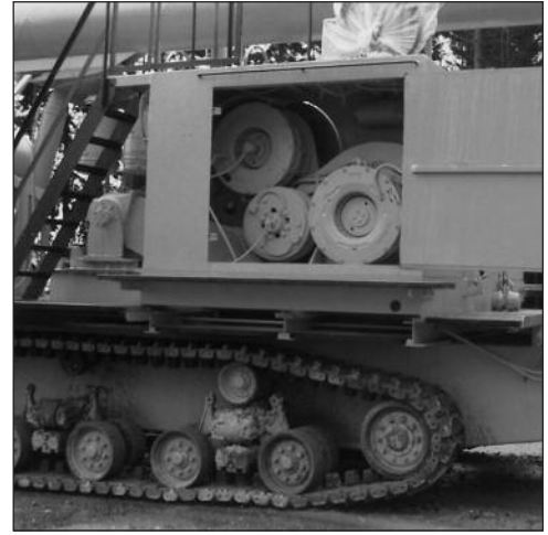
Wichita Kopper Kool Brakes provide precise tension control on winch drives for mobile equipment.
