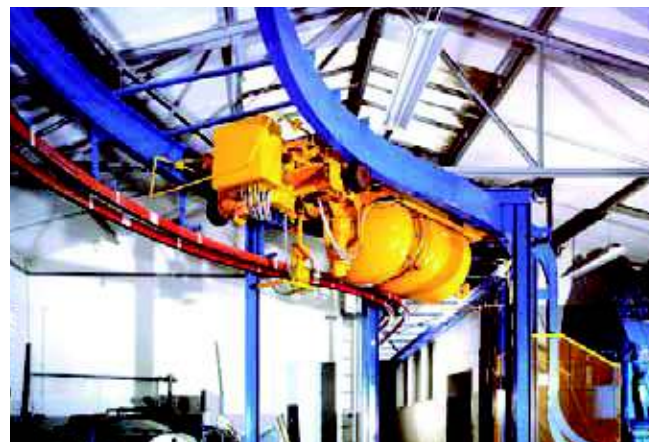
Feed and control of a concrete skipper
