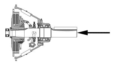
**5.9** The operating handle (hand lever) may be installed on either side of the PTO engagement shaft, depending upon space requirements and convenience to the operator. Install lever with the cast hex facing away from the PTO.
