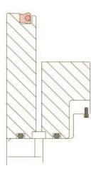
7.2.6 Liberally lubricate all seals and seal surfaces with clean hydraulic oil prior to assembly. Insert the **piston (5)** into the **cylinder (2)** while taking care not to damage the seals.
